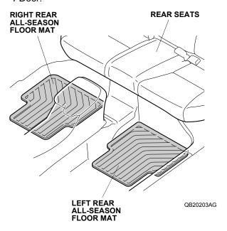
2-Door: Install the ring in the right rear all-season floor mat over the anchor. Push on the ring into the anchor to secure the retaining tabs, then turn the knob on the anchor 90° to secure the right rear all-season floor mat.
